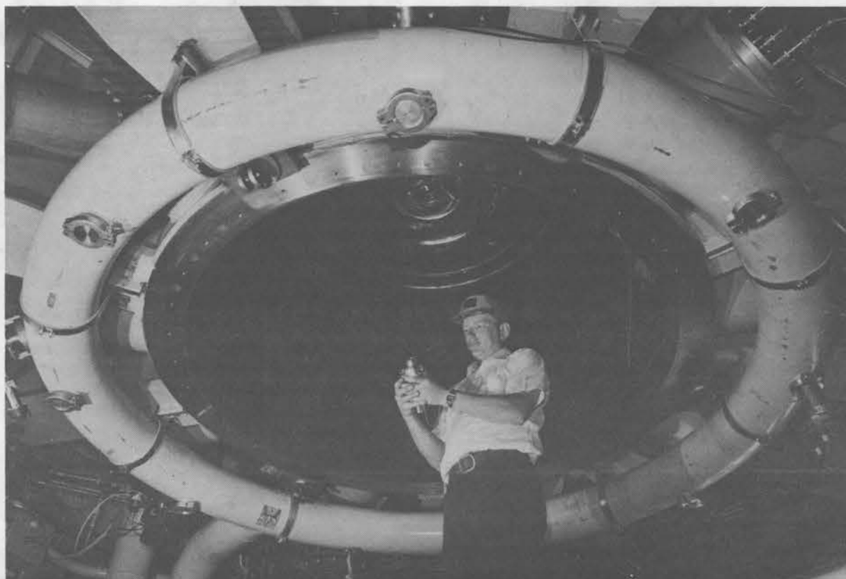
FAST GAS VALVE and supersonic injection nozzle that Rick Spielman (1273) is holding are part of the gas-puff system used to produce soft x rays on Sandia's Saturn accelerator. Rick is standing underneath the center of Saturn. The large, light-colored ring is the vacuum manifold through which Saturn's center is evacuated before each shot.
